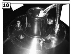
Place motor cover over 3 screws and twist cover into position. Take 3 screws removed earlier and replace, tighten all 6 screws securely.
